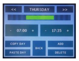
Each schedule component has a boolean 'out' slot that will be true when the actual time is within one of the set periods. This can be linked to logic to command equipment on/off. 23.5 °
