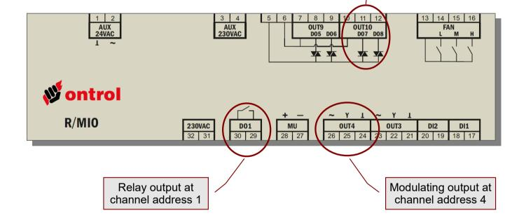
For add-on relay modules, channel addresses are:
