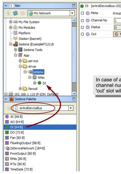
In case of an invalid channel number, the 'out' slot will be null.
