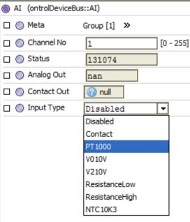
In case of an invalid channel number, the 'out' slot will be nan or null.
